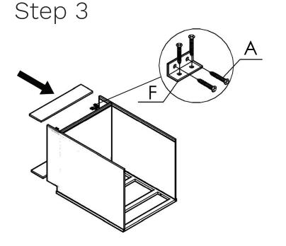
3. Place the small toe kick into the grooves below the floor board on the back side of the cabinet (opposite of face) paint side out. Slide the large toe kick into the grooves below the floor board on the front side. Place one metal clip on the inside of each corner below the floor board. This will connect the large and small toe kicks to the left and right sides of the cabinet.
