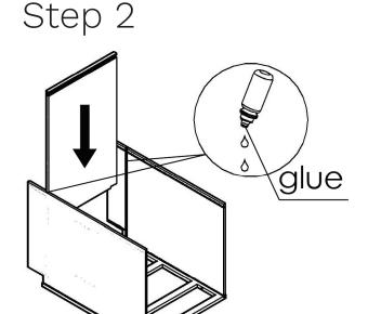
2. Slide floor board into the parallel grooves on the walls. Make sure the floor board notch fits into the grooves on the face frame. Make sure the groove on the floor board is inward toward the inside of the cabinet.
