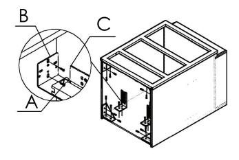
5. Locate L brackets and match the holes on the brackets to the corresponding holes on the inside of the back wall. Use small screws to attach them to the cabinet. There are six L brackets in total.
