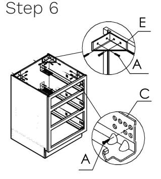
6. Place one corner bracket into each corner on the inside of the cabinet. This will secure the face frame and back wall to the left and right sides of the cabinet.
