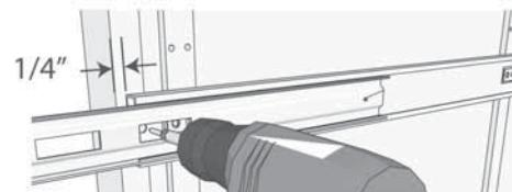
5. Attach slide to face frame (or side wall) of cabinet with front of slide 1/4" back from outside front of cabinet as shown with 1/2" wood screw.
