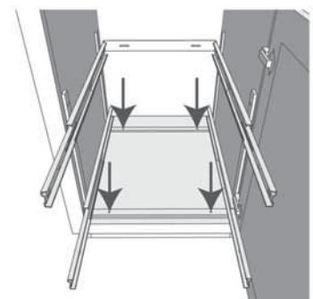
6. Attach U-shaped support brackets to the cabinet floor with the mounting holes 1-13/16" back from outside front of cabinet as shown with 3/4" wood screws.
