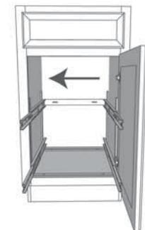
4. Place frame inside cabinet and position frame adjacent to side of cabinet opposite from the hinged door to allow baskets to slide out without obstruction.
